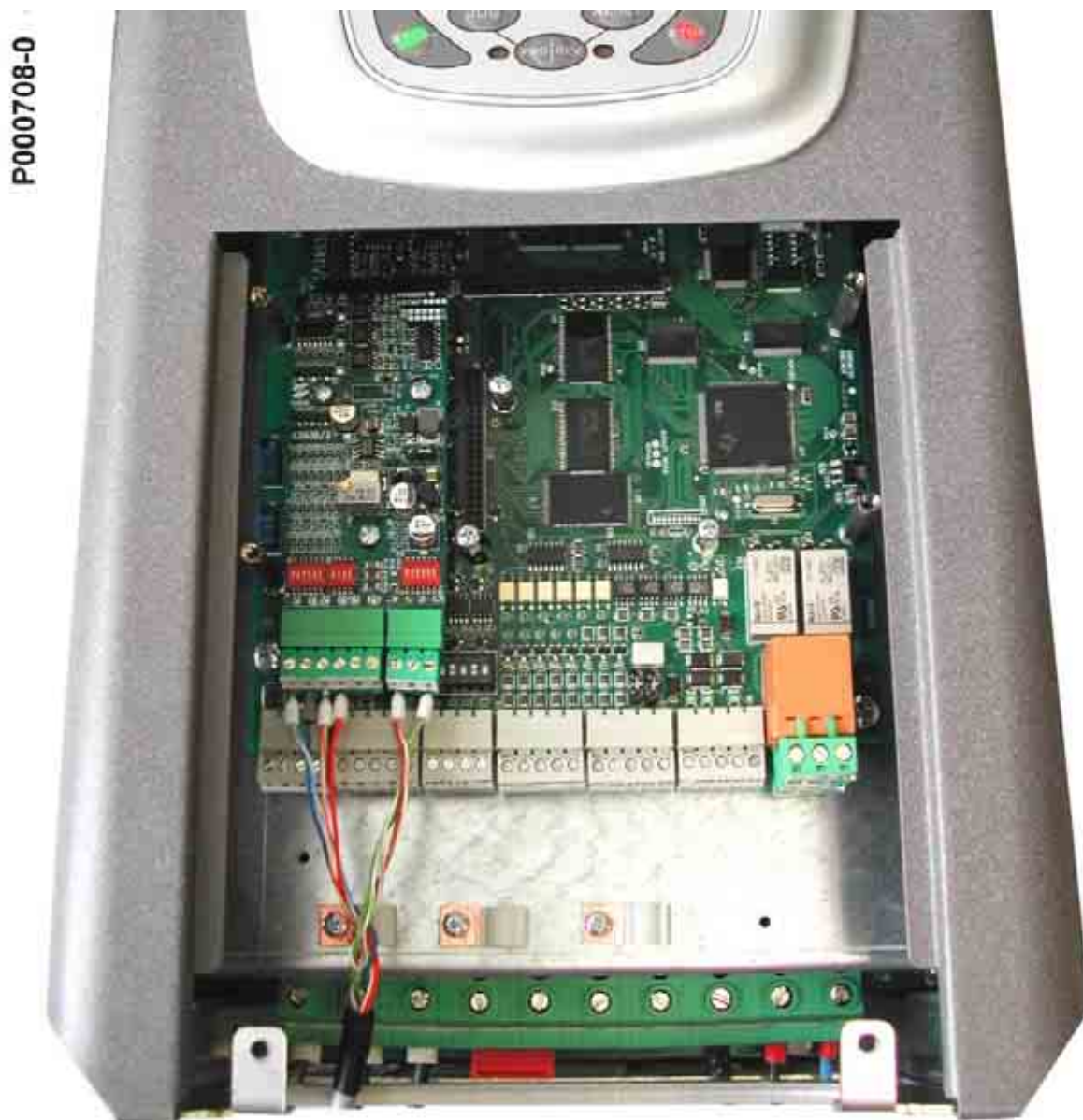
Figure 104: Wiring the encoder cable
