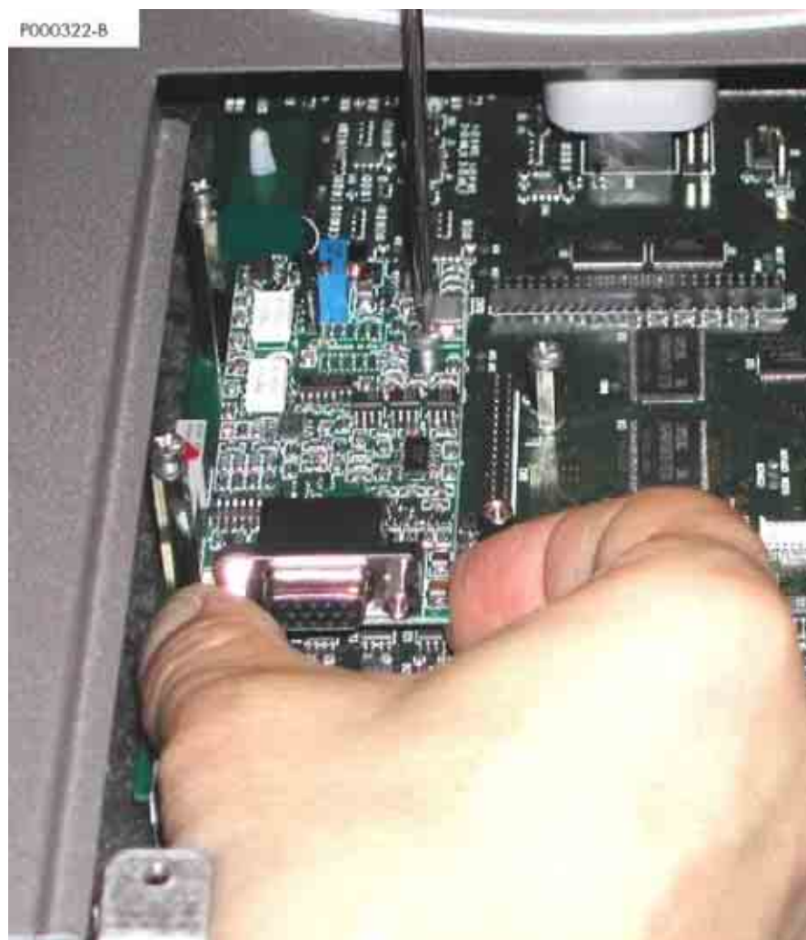
Figure 148: Fitting the ES860 Card inside the Inverter
