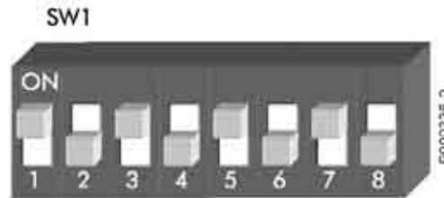
Figure 151: Dip-switch SW1 setup for Three-channel Mode reception
