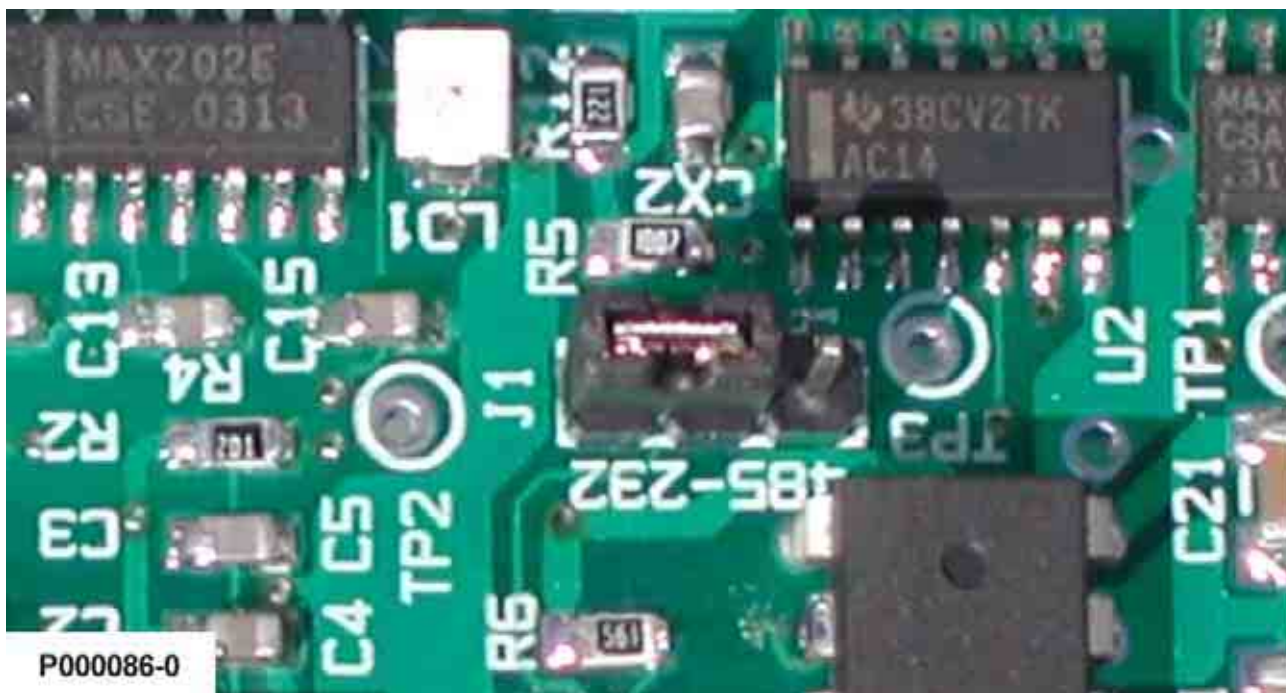
Figure 107: Jumper setting RS232/RS485
