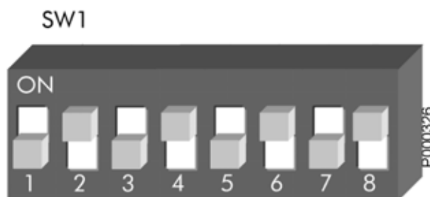
Figure 153: Dip-switch setup for Five-channel Mode reception
