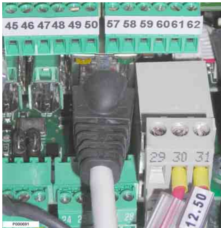
Figure 145: Wiring the Ethernet cable
