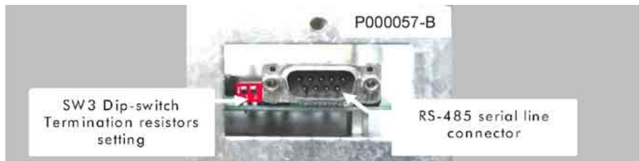
Figure 45: Gaining access to dip-switch SW3 and connector RS-485 (SINUS PENTA S05 to S20)
