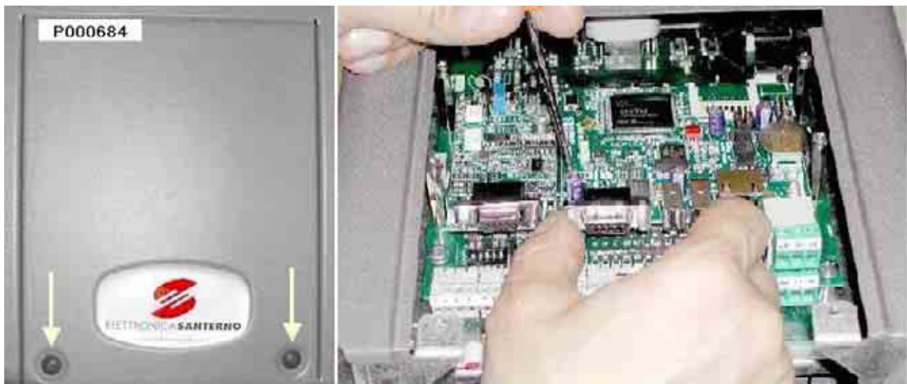
Figure 141: Data Logger board fastened to its slot (Slot B)
