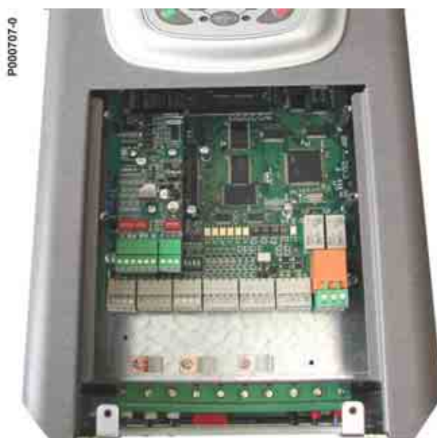
Figure 98: Encoder board fastened to its slot
