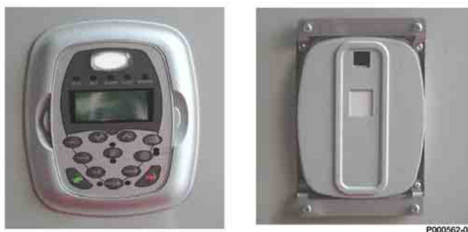
Figure 62: Front/rear view of the display/keypad and its shell.
